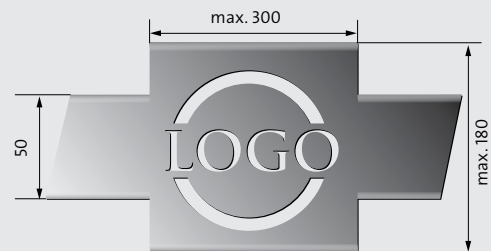
Clearance (lasered area): max. 10 mm
